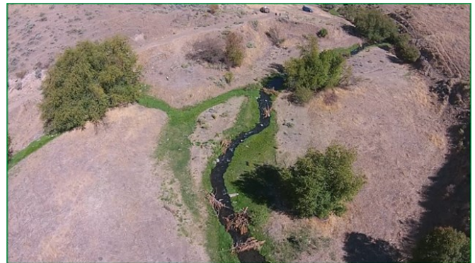
September 10th, 2015 Post-Project Flight after Post Assisted Log Structures installation and structures are slowing water habitat and PALS may have increased ground water storage by holding water behind structures. The floodplain area has better hyporeic connection and has greened up substantially in the month after project implementation.
