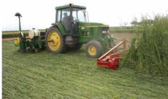
Figure 16.7. Roller-crimper creates a weed-suppressing cover-crop mat through which it is possible to plant seeds or transplants. Here cotton is being planted behind rye that has been traveled over by the roller-crimper. Photo by Jeff Mitchell.
